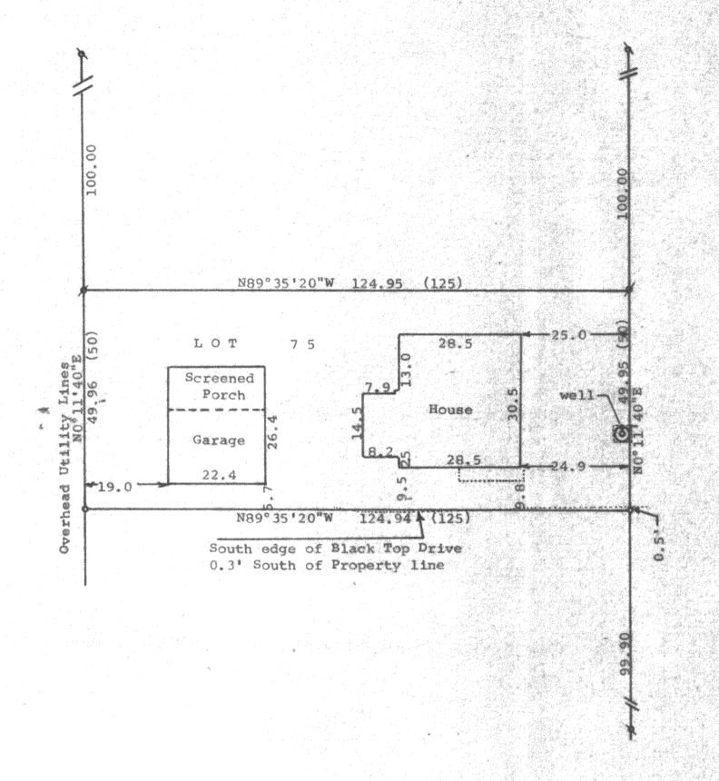
Scale - 1" = 20" #= 14" Iron Pipe Found o = 14" X 24" Iron Pipe Set W = 3/4" Iron Pipe Found (0.00) = recorded distance Bearings referenced to the recorded bearing of N89°35'20"W along the north line of Lake Delayan Highlands. Owners: Clifford V. and LaVerne M.
